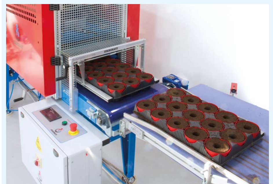
NIR connected in line with a RW transplanter.
