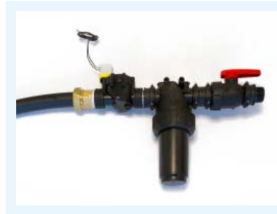
Water distribution group 1¼" for recoiling system and 1" for suspended or ground hose: ball selector valve, net filter and solenoid valve.
