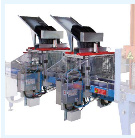
ND with 4 label machines mod. ETC for applying approx 3200 labels/hour.
