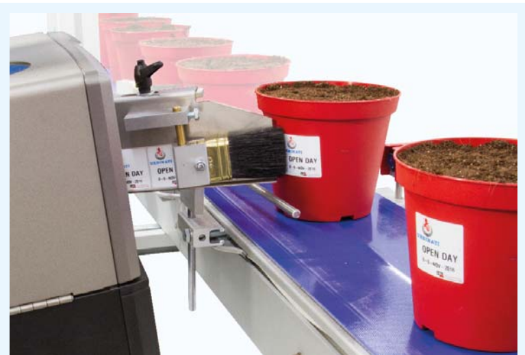
Labelling machine mod. ETS : applies 40x40 mm labels on single pots .
