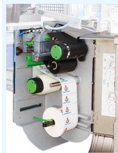
Printing head completely openable for easy loading.
