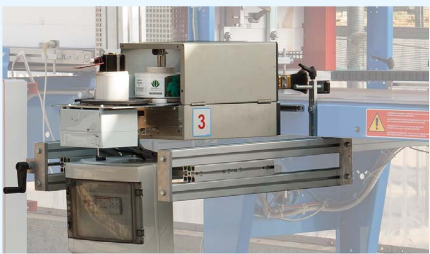
Labelling machine mod. ETS : applies 70x220 mm labels on the tray side .
